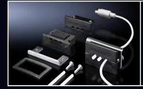
Connector gland, small Whatever the surface, this component makes light work of introducing pre-assembled cables. Installation is possible up to a material thickness of 4 mm. Cables can be securely fastened to the integrated strain relief component using cable ties.
